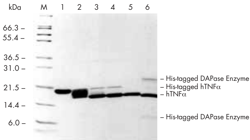
Figure 5. Removal of the His tag from His-tagged hTNF \alpha using the TAGZyme System.
